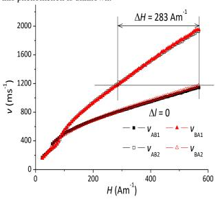
Figure 2 Domain wall velocity with unidirectional effect (FeSiB) [25].
