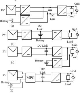
Fig. 1. Basic topologies for photovoltaic and energy storage, [1], [2], [5]-[27],
