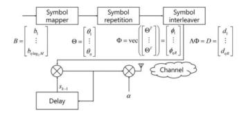
Fig. 1 Differential phase shift keying modulator system model
