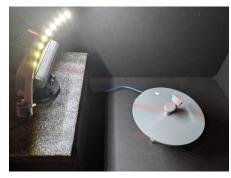
Fig. 3: Photograph of the constructed rotary 3D scanner. The left side shows a 2D camera (PS3 Eye) with a mounted line laser and an LED strip. The other side contains the rotary table driven by a stepper motor.
