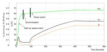
Figure 3 Simulation of the turbine's start up, synchronization (phasing) and its power control [11]
