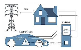
Fig. 4 Vehicle-to-Grid (V2G) system [6]
