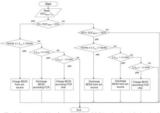
Fig. 3 Control algorithm for maintaining SOC by charging / discharging in the dead band
