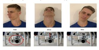
Figure 2 Gymbal control on drone
