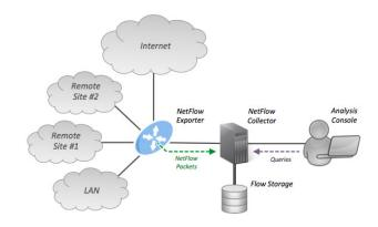
Fig. 1. Typical connection of NetFlow collector
