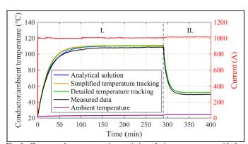
Fig. 1. Current and temperature time variations during measurement with the conductor 429-AL1/52-ST1A [4].
