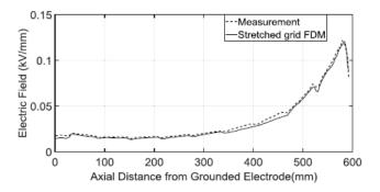
Fig. 4 Comparison of the measured and calculated electric field, [17].
