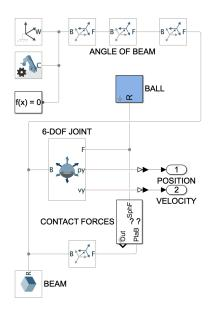
Fig. 3. Simscape model of Ball and Beam with rolling
