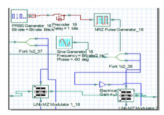
Fig. 2 DPSK modulation scheme in Optisystem
