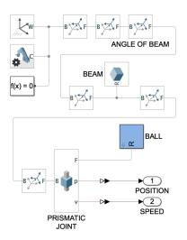
Fig. 2. Simscape model of Ball and Beam without rolling
