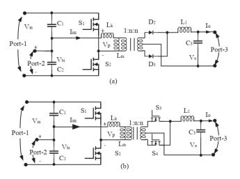
Fig. 2. Isolated topology with two ports, [18], [20], (a) Primary freewheel
