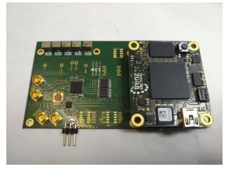
Fig. 2: Designed data acquisition board with custom made ASIC AD converter
