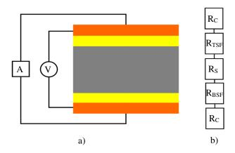
Fig. 2 Principle of the measurement of the solder joint's electrical resistance a) and it's alternative resistor model b)
