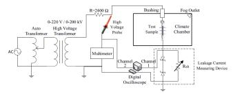
Fig. 2 Schematic diagram of the experimental set-up, [9].
