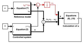
Fig. 1. Block diagram of the proposed controlled system.
