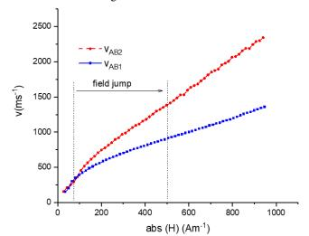
Fig. 2 Velocity versus magnitude of the applied field for sample with unidirectional effect (fast wall  $v_{AB2}$ , slow wall  $v_{AB1}$ ). DW propagates along the same path and in the same direction (where indexes A, B correspond to the ends of the sample) but it is driven by opposite field.
