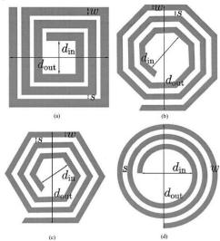
Fig. 3 Type of inductor realization: (a) square, (b) hexagonal, (c) octagonal, (d) circular [2]
