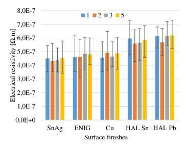
Fig. 3 Graphical representation of the average values of electrical resistivities of the solder joints after 1, 2, 3 and 5 reflows
