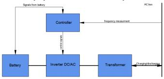
Fig. 1 Block diagram of the model
