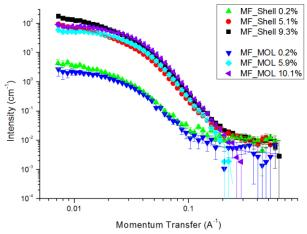
Fig. 2. SANS data (points) and fit (curves) for the ferrofluids based on insulating transformer oils SHELL and MOL with different magnetic mass fraction of NPs.
