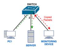
Fig. 2. Connection of NetFlow probe in infrastructure
