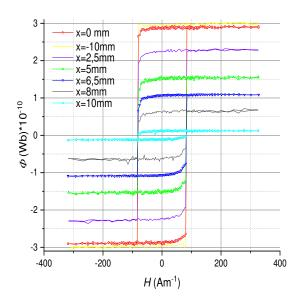
Figure 6 Measurement of hysteresis loops on different parts of the sample.
