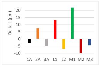
Fig. 2 Comparison of irreversible dimensional change of sample after heating and cooling cycle.
