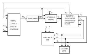
Figure 1 Block diagram of a Small Hydropower Plant [13]
