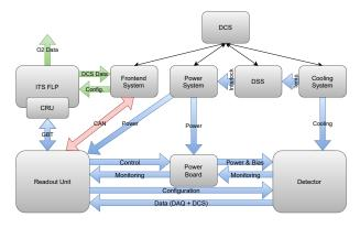
Fig. 2. DCS architecture of the ITS detector
