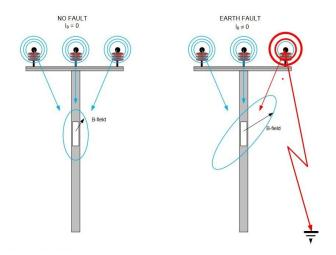
Fig. 4. Comparison of the change of the magnetic field in normal operation (left side) and in the fault state (right side) [13].
