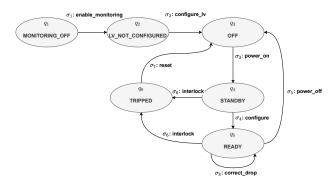
Fig. 3. FSM model for the HIC unit within the central DCS
