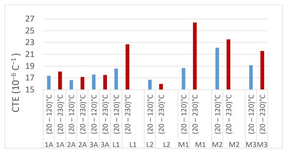
Fig. 1 Coefficient of thermal expansion in "Y" direction below and above Tg.
