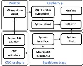
Fig. 1 The system diagram
