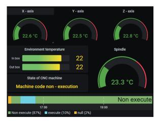
Fig. 5 Visualization of the current state of temperatures and machine operation (part C)
