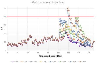
Fig. 1. Graph of maximum currents in the network[4].
