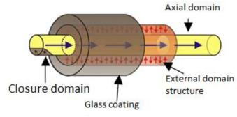
Figure 1 Schematic domain structure of amorphous glass-coated microwire with positive magnetostriction [8].
