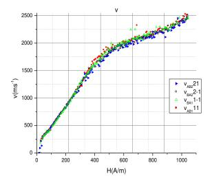
Figure 3 Four different velocities of a domain wall moving without unidirectional effect (Fe42.5Co35Si7.5B15).
