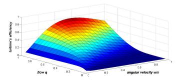
Figure 5 The efficiency of the hydraulic turbine  $(R_{blades} = 1.9 \text{m} \text{ and } A_{blades} = 8 \text{m}^2) - \text{Maximum turbine's}$  efficiency is approx. 77% [14]
