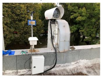
Figure 6 Weather monitoring station together with FSO head and RF line.
