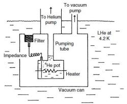
Fig. 4. A continuously operating  $^4\text{He}$  refrigerator for the temperature range between 1.3 K and 4.2 K. [11]
