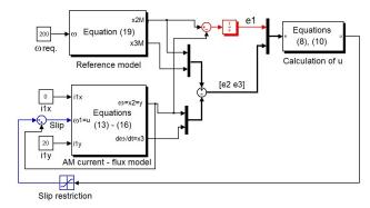
Fig. 3. Block diagram of induction motor control.
