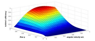
Figure 4 The efficiency of the hydraulic turbine  $(R_{blades} = 1.9m \text{ and } A_{blades} = 9m^2) - Maximum turbine's efficiency is approx. 88% [14]$
