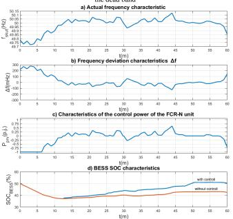
Fig. 4 Characteristics of a) actual frequency, b) frequency deviations, c) control power of PRV unit, d) charge level BESS (with and without SOC maintenance) for a time interval of 60m
