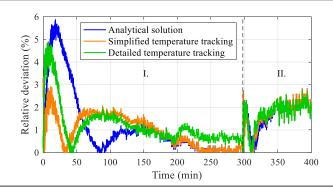
Fig. 3. Relative deviation from measured data for conductor 352-AL1/59-ST1A [4]
