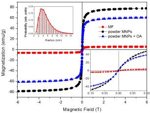
Fig. 1. Magnetization curves of the powder magnetite NPs, NPs with surfactant and MF. Inset 1 (left upper corner): distribution of MNPs in MF calculated from the magnetization. Inset 2 (right bottom corner): superparamagnetic behavior (zero hysteresis) of the samples.
