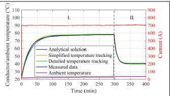
Fig. 2. Current and temperature time variations during measurement with the conductor 352-AL1/59-ST1A [4].
