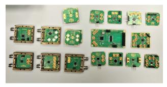
Fig. 1: Several types of designed front-end UWB ASIC circuits assembled on evaluation PCB boards
