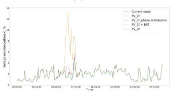
Fig. 4. Graph of voltage unbalance factor after installing 30% PV in Grid
