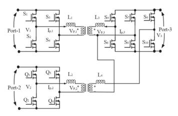
Fig. 4. Triple port active bridge converter based on dual transformer [28] and [29]
