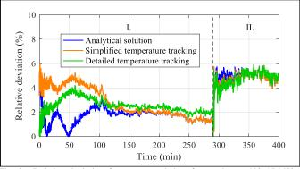
Fig. 3. Relative deviation from measured data for conductor 429-AL1/52-ST1A [4]
