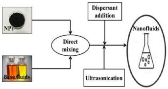
Fig. 1. Preparation of nanofluid [21].
