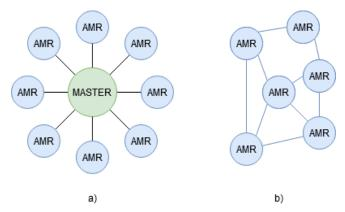
Fig. 4. a) centralized, b) decentralized arhitecture of fleet management system.
