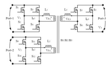
Fig. 3. Isolated triple active full bridge converter [25]-[27]
