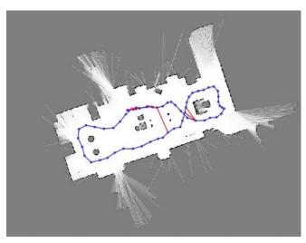
Fig. 3. Occupancy grid created by lidar SLAM.
