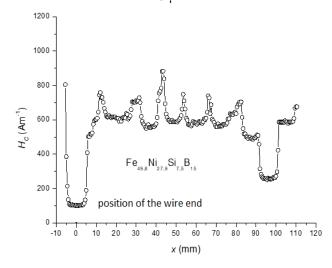
Figure 4 Distribution of local critical (nucleation) fields along the microwire (x - distance between the wire end and the center of the magnetized coil) [26].
