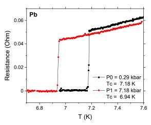
Fig. 6. Superconducting phase transition of lead at atmospheric pressure and under pressure of 7 kbar in piston cylinder cell.
