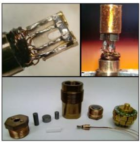
Fig. 5. Piston cylinder cell from Centre of Low Temperature Physics, Slovak Academy of Sciences in Košice. Top pictures shows detail on sample, which maximum dimension is about  $350\mu m$  on bottom picture is disassembled whole piston cylinder cell.
