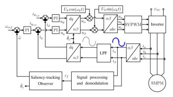
Fig. 2. Block diagram of rotating HF sinusoidal signal injection based method.
