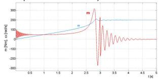
Fig. 2. Time responses of mechanics characteristics of the motor model at suplying by current vector.
