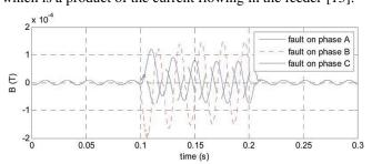
Fig. 5. Measured magnetic fields along different axes under single-phase short-circuit conditions. The figure shows the magnetic-field waveform along the x axis [14].
