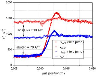
Fig. 3 Position dependencies of DW velocities for DW propagating in homogeneous field (empty symbols) and for DW, that propagates in inhomogeneous field jump from 70A/m to 510 A/m (full symbols).
