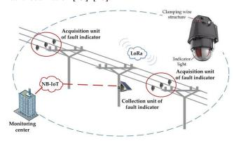
Fig. 6. The working principle of fault indicator based on LoRa and NB-IoT [16].
