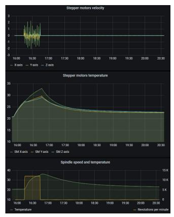
Fig. 3 Graphs of temperatures and speeds of CNC machine drives (part A)
