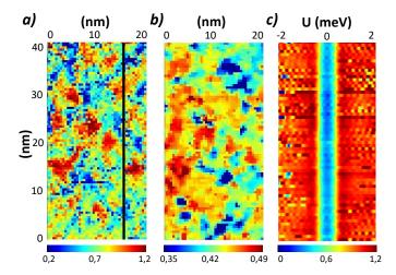
Fig. 2. (a) STM surface topography of a  $20 \times 40 \text{ nm}^2$  surface area at 500 mK. (b) superconducting energy gap map obtained from tunneling spectra measured at each point of the topography from (a). The top view of the tunneling spectra measured along a 40 nm long line plotted in Fig. (a) in a voltage window  $\pm 2 \text{ meV}$  in the marked colour scale is shown in (c).
