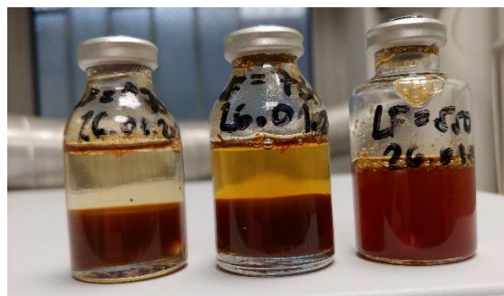
Fig. 5. The final product of the synthesis: magnetoferritin colloidal solution with protein concentration with loading ~ 550 Fe atoms per the one protein biomacromolecule; and higher iron loading ~ 730 Fe atoms per the one protein biomacromolecule; and the highest iron loading ~ 810 Fe atoms per the one protein.
