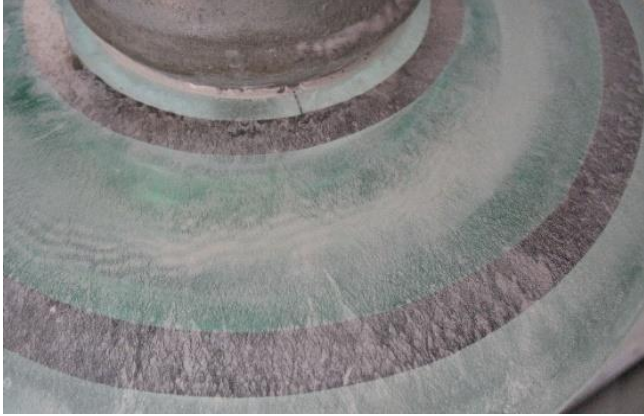
Fig. 1 Electrodes made of conductive paste applied to the surface of the glass insulator.
