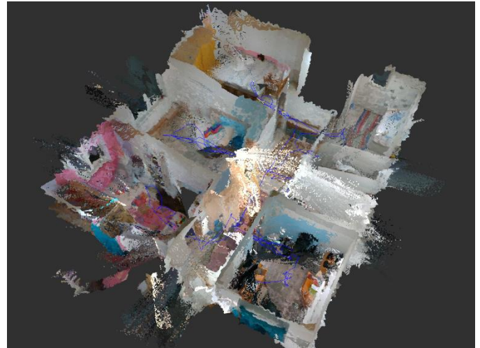
Fig. 2. Point cloud created with 3D scanner in indoor environment.
