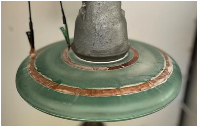
Fig. 2 Copper tape electrodes on a glass insulator during measurement.
