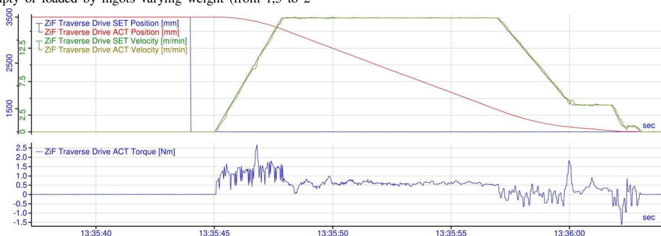
Fig. 3 Velocity, Position and Torque profiles during positioning of Ingot Feeder Unit (traverse drive)
