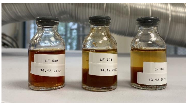
Fig. 1. The final product of the synthesis: magnetoferritin colloidal solution with protein concentration with loading ~ 550 Fe atoms per the one protein biomacromolecule; and higher iron loading ~ 730 Fe atoms per the one protein biomacromolecule; and the highest iron loading ~ 810 Fe atoms per the one protein.
