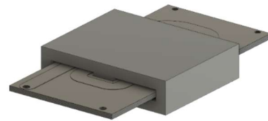
Fig. 2 3D model of designed planar transformer
