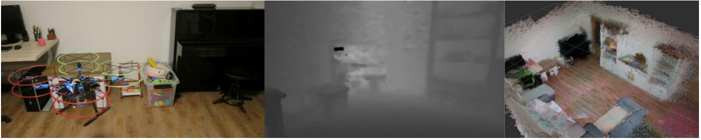
Fig. 2 From left to right. Flying a drone in the room. Output from a depth camera. Captured point cloud from the room.
