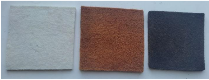
Figure 1. Examples of native felt, felt modified with 20% ferrous sulfate solution and magnetic iron oxide particles modified felt (from left to right).
